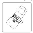
Remove batteries from remote control
